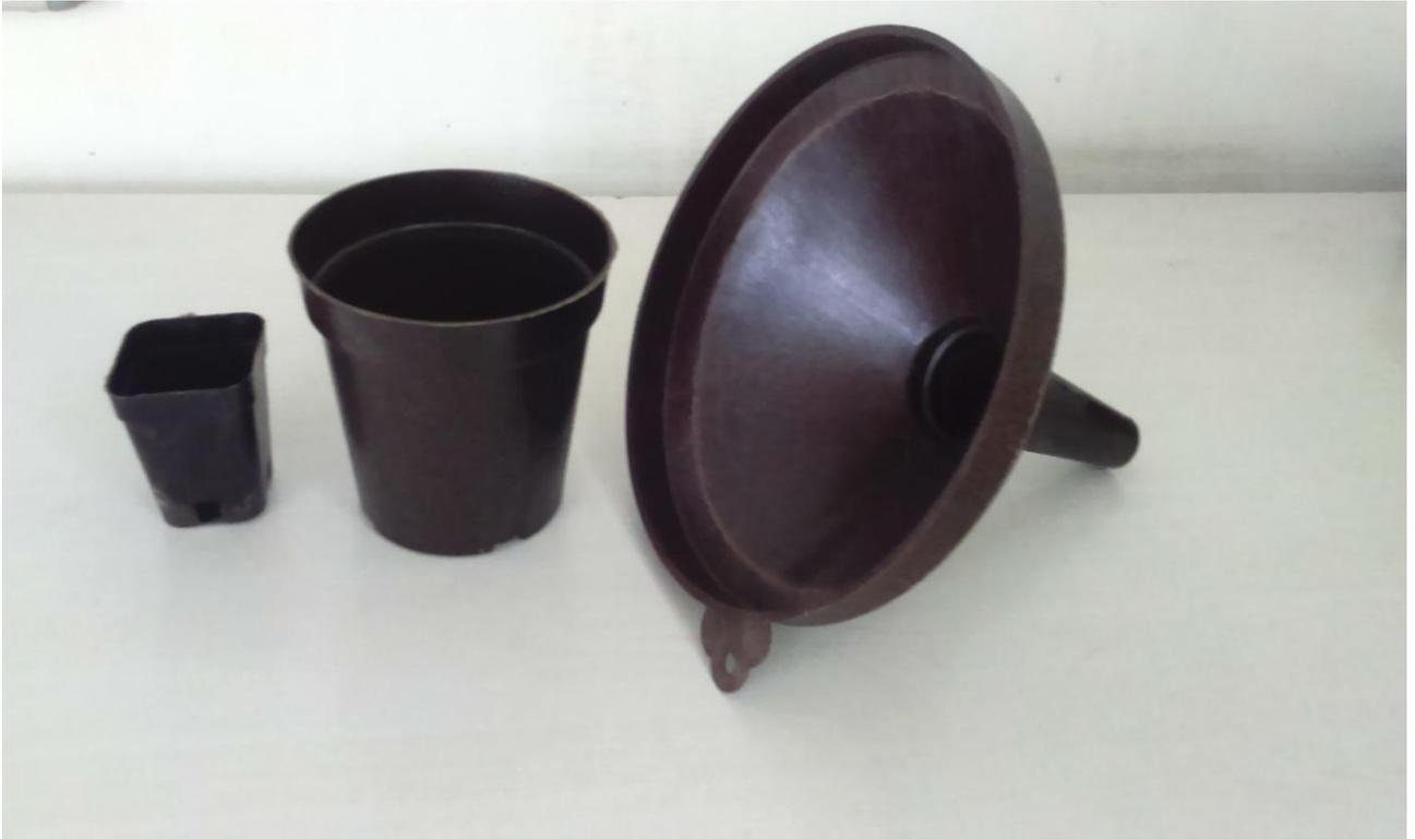
Figure 3.19 PP-Coir Biocomposite Products
