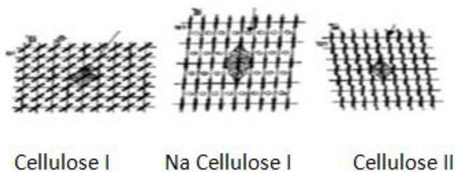
Figure 2.4 Influence of alkali treatment on cellulose structure
