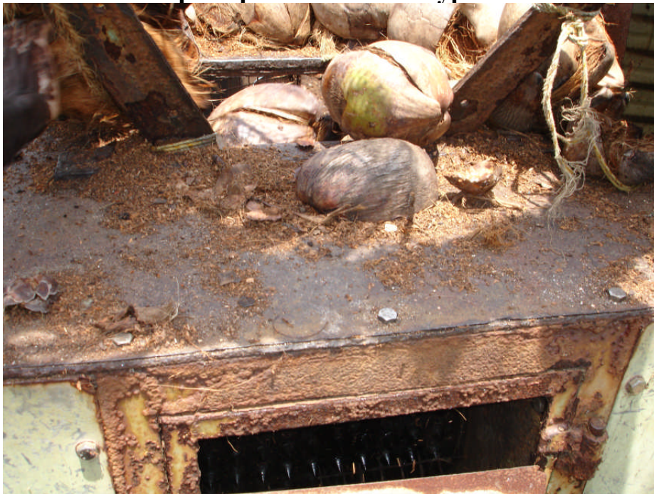
Fig.1 (a). A view of the crusher used to crush the Coconut husk
