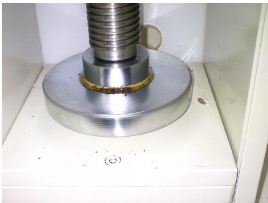
Fig.3 Oil recovery from the coir pith
