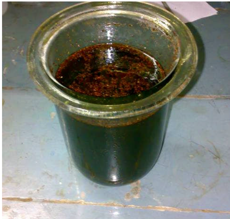
Fig.6. Oil extracted from the coir pith using the screw press
