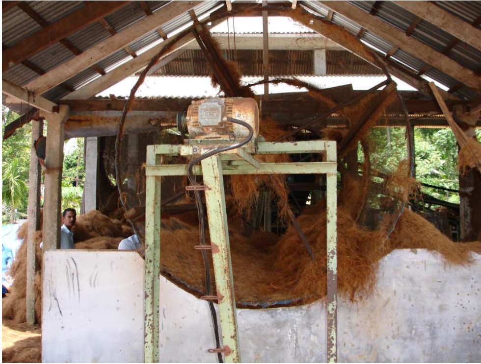
Fig 2(a): A Rotating mesh screen separating the coir and coir pith
