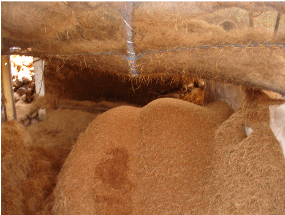
Fig 2(b): Coir pith is collected from the bottom of the screen.
