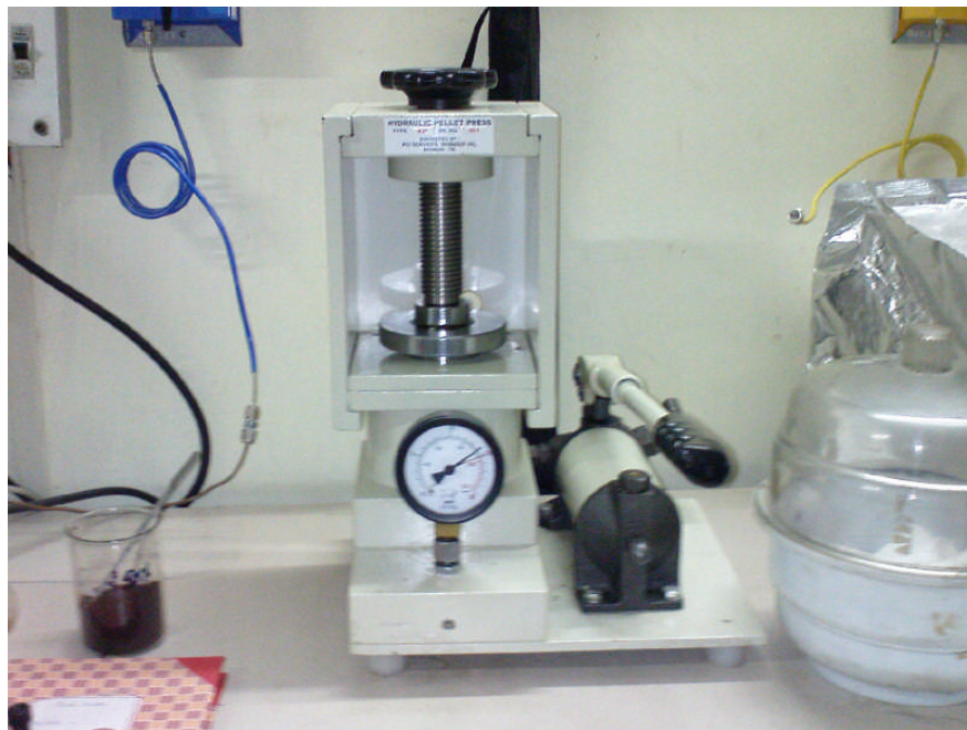
Fig.2. Hydraulic press used during experiment
