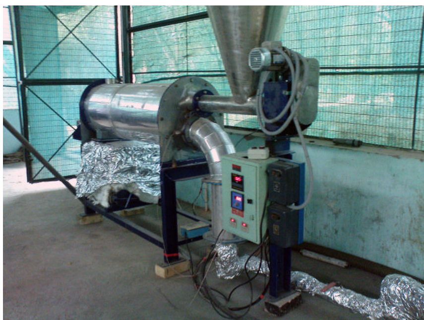
Fig.2: View of a pyrolyser reactor (proto type) used for conversion of biomass in to liquid fuel
