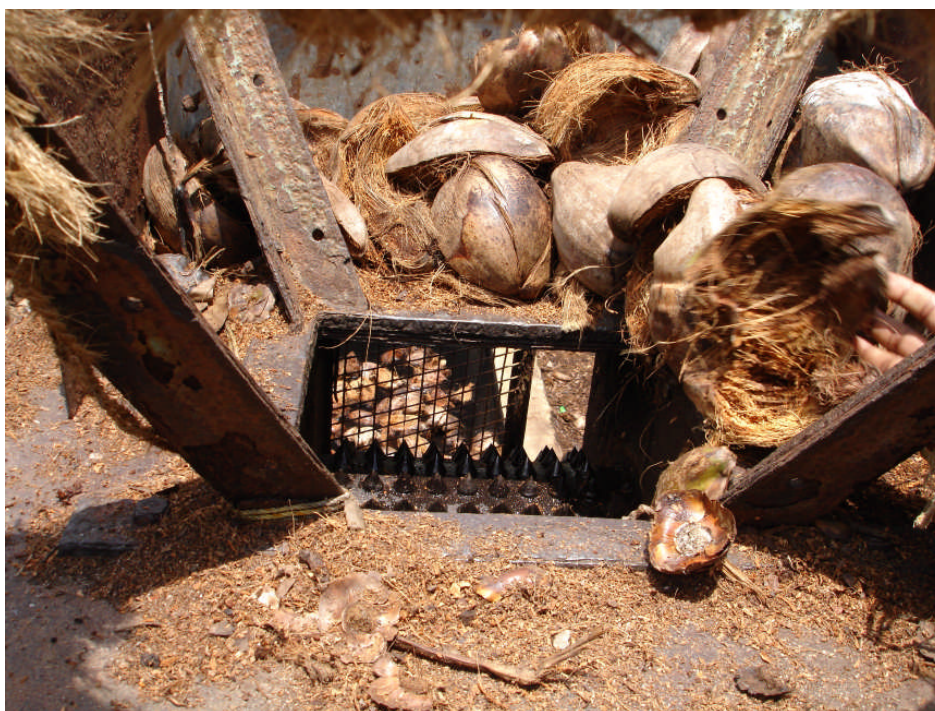
Fig.1 (b). The inner view of the coconut husk crusher
